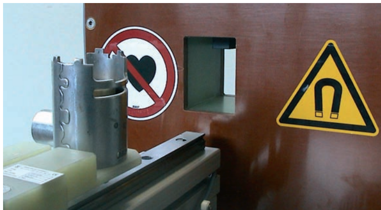
A rectangular axial coil (RAB) used to magnetize a small 2-poles motor
