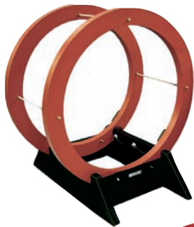
Round, Single Helmholtz For susceptibility testing
